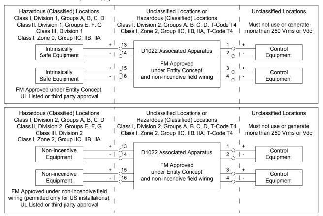
Non-incendive field wiring is not recognized by the Canadian Electrical Code, installation is permitted in the US only.
