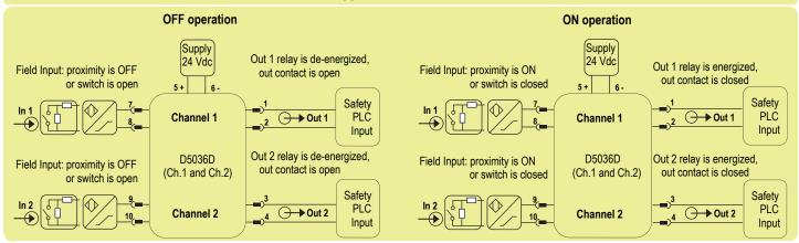
**Description:** For this application, enable input line fault (open or short) detection and direct input to output transfer function, by set the internal dip-switches in the following mode (see page 9 for more information):
