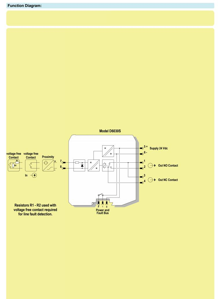
Relay contact shown in de-energized position. Terminals 1-2 open, terminals 3-4 close.
