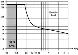
Mechanical / Electrical life: 5 \* 10<sup>6</sup> / 3 \* 10<sup>4</sup> operation, typical. Operate / Release time: 8 / 4 ms typical. Bounce time NO / NC contact: 3 / 8 ms typical.
