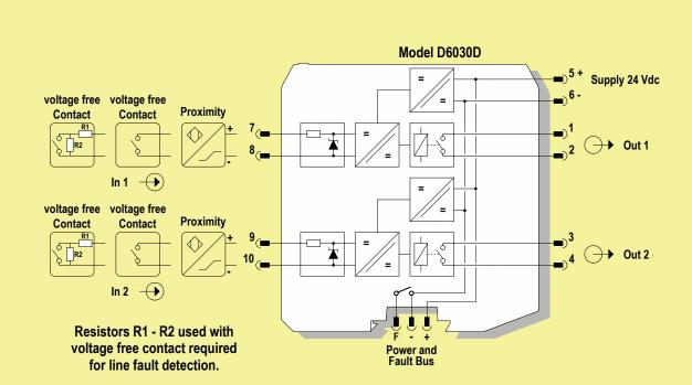
Relay contact shown in de-energized position. Terminals 1-2 and 3-4 open.
